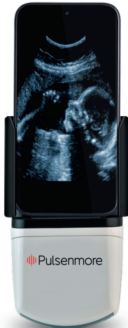
Figure 3 The Pulsenmore ultrasound device produced by GE Healthcare. Reproduced with permission from GE Healthcare.
